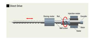
Fig. 10 Drive Mechanism of Injection Screw
