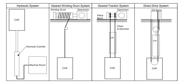
**Table 2 Lift Mechanisms of Residential Elevators**
