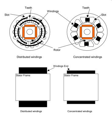
Fig.4 Stator Core Construction
