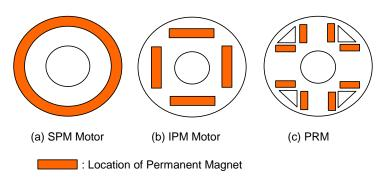
Fig.1 Rotor Construction of Permanent Magnet Motor
